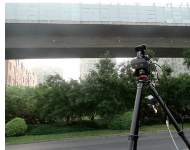
(b) 桥梁挠度测试 (b) Deflection test
