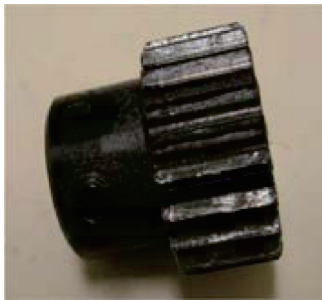
图13 磨损的太阳轮 Fig.13 Wear sun gear
