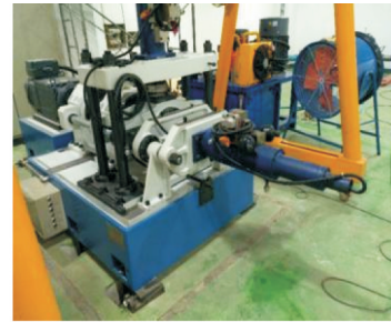
(a) 高铁轴承综合试验台 (a) High speed railway bearing test bench
