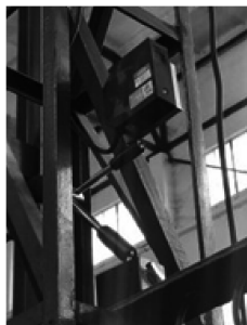
(a) 激光位移传感器测点布置 (a) Layout of measuring points of laser displacement sensor
