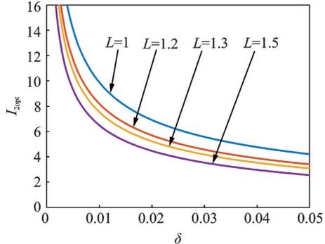
(b) LISD2中最优性能指标与 $\delta$ 的关系(b) Relationship between the optimal performance index and  $\delta$  of LISD2图8 LISD中最优性能指标与 $\delta$ 的关系Fig. 8 Relationship between the optimal performance index and  $\delta$  of LISDs
