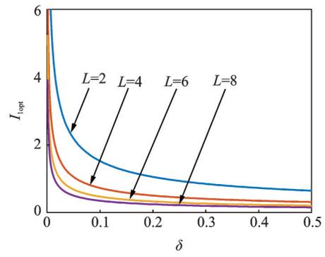
(a) LISD1中最优性能指标与 $\delta$ 的关系(a) Relationship between the optimal performance index and  $\delta$  of LISD1
