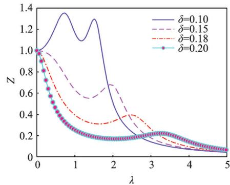
(b)  $L=2.1$ 时,不同 $\delta$ 下LISD2主系统幅频曲线(b) The amplitude-frequency curves of LISD2 with different inerter-to-mass ratios  $\delta$  at  $L=2.1$ 图7 不同 $\delta$ 下LISD主系统幅频曲线Fig. 7 The amplitude-frequency curves of LISDs with different inerter-to-mass ratios  $\delta$
