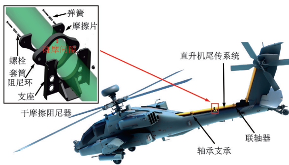
图 1 某装有干摩擦阻尼器的武装直升机尾传动系统 Fig. 1 TRDS in an armed helicopter equipped with a dry friction damper
