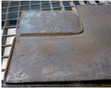
(c) 轨道垫板挤压及磨损 (c) Squeeze and wear of track pad
