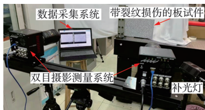
(a) 基于高速摄像的振动位移测量试验 (a) Vibration displacement measurement test based on stereo-cameras
