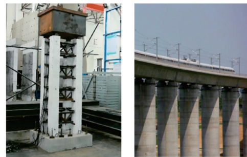
(a) 铁路屈曲支撑桥墩振动台试验 [12] (b) 铁路圆端型实体桥墩 [13] (a) Shaking table tests of railroad buckling support pier [12] (b) HSR-RERSCSS concrete pier [13]
